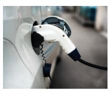
Depending on the battery technology in your vehicle, Level 2 charging generally takes 4 to 6 hours to completely charge a fully depleted battery. Today Level 2 charging is the most widely used medium for vehicle charging.
